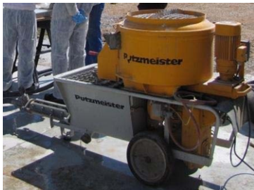
Typical pumping and mixing equipment
